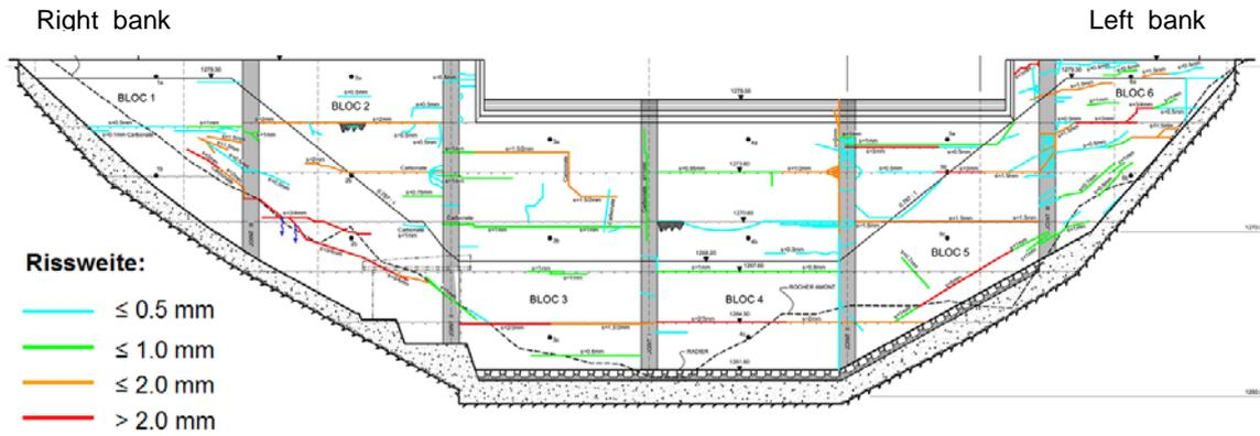
**Figure 14:** Concrete expansion in the old Sera Dam. Fissure pattern (structural cracks) is very similar to the one at the Zeuzier arch Dam (cracks following valley shape on the downstream face).
