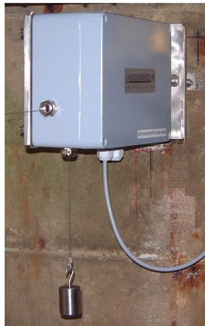
**Figure 63:** Continuous temperature and relative humidity measurements - invar wire deformation measurements.
