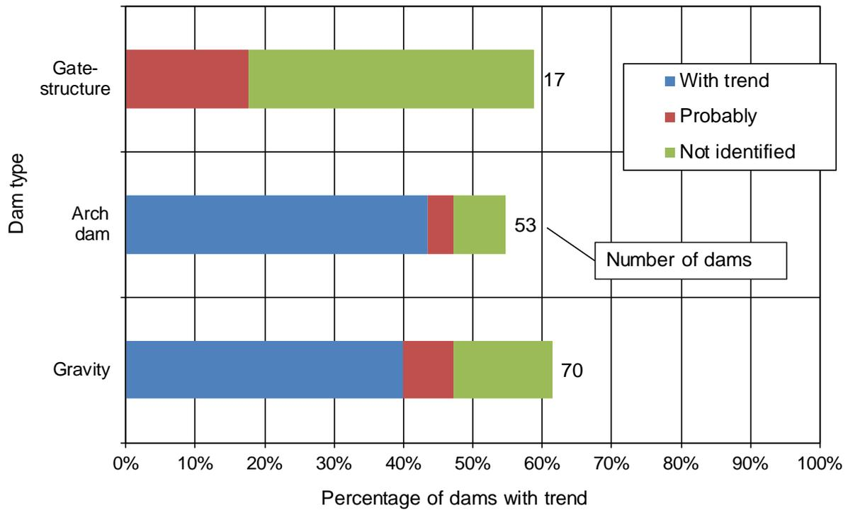
**Figure 33:** Percentage of affected dams according to trends, depending on dam type.
