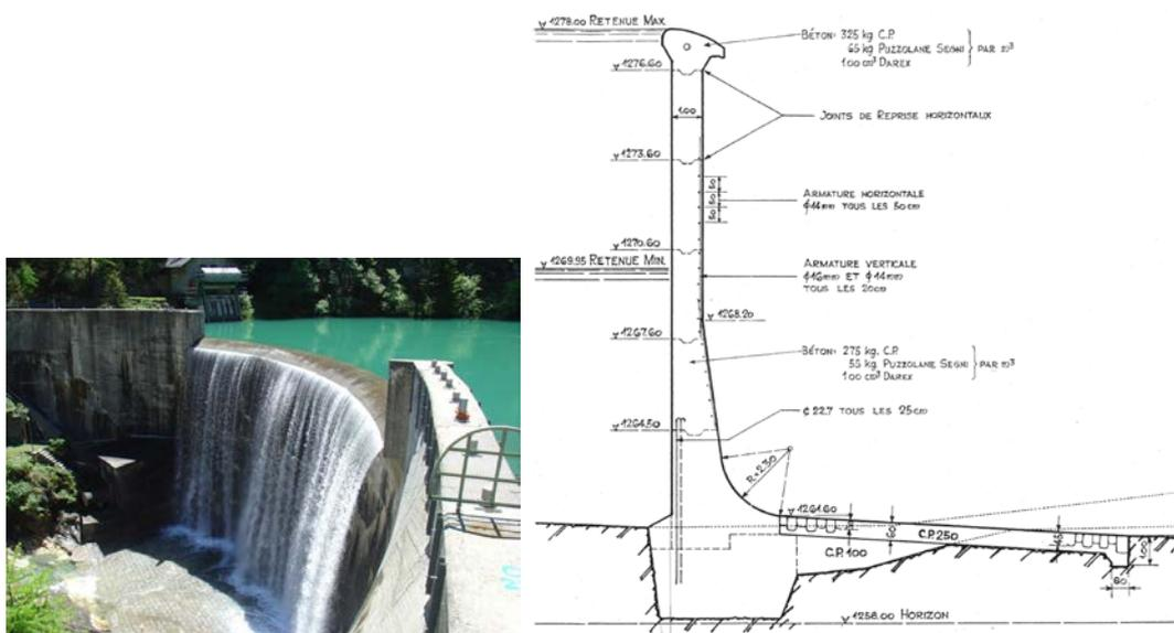
**Figure 66:** Sera Dam – cross section
