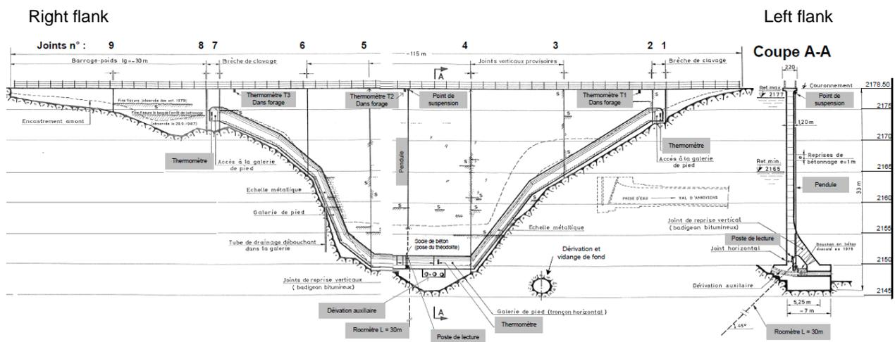
**Figure 55:** Downstream view of the dam – Vertical cross section.
