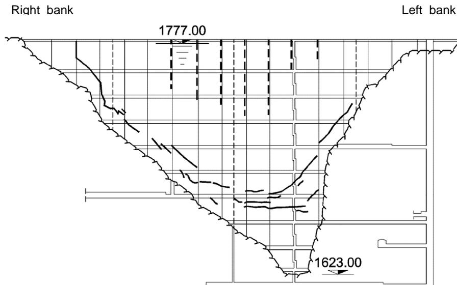
**Figure 15:** Crack pattern at Zeuzier arch Dam following valley closure
