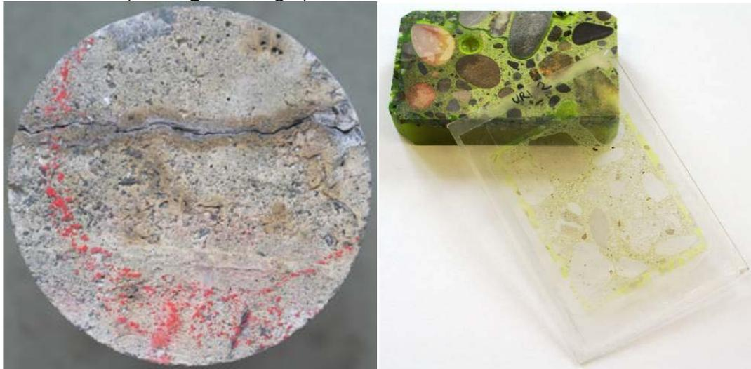
**Figure 6:** Surface of a drill core  $d = 100$  mm with cracks due to AAR (left) and concrete sample  $50 \times 90$  mm with impregnated thin section / thin section for observation under the light microscope (right) [10].
