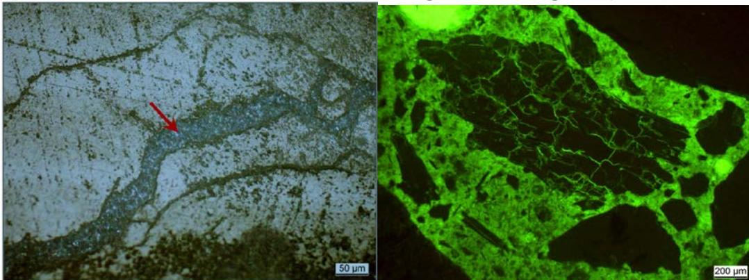
**Figure 8:** Micro crack filled with AAR-generated products in an aggregate grain (left, microscope image of a freshly ground moist concrete surface before impregnation) and aggregate grain containing multiple micro-cracks (right, microscope image with fluorescent light) [10].
