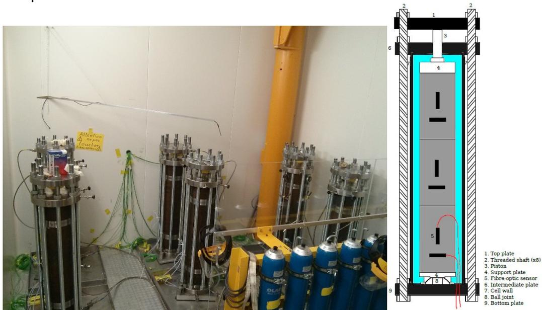
**Figure 4:** Test rig for AAR swelling simulations on concrete cylinders with 3d compressive load (left) and schematic of the 3d load cell with fiber optic strain measurement (right) [8].
