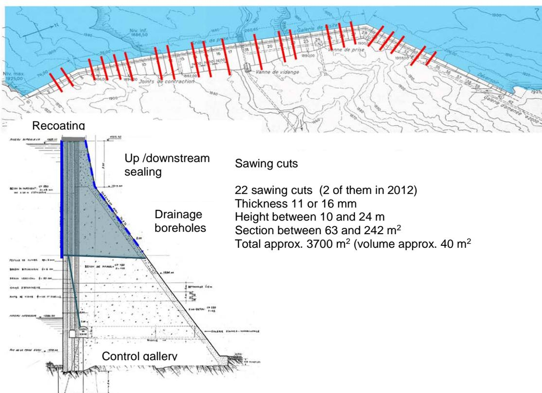
**Figure 79:** Plan view of saw cuts - typical cut.
