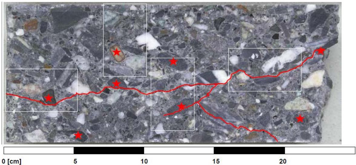
**Figure 7:** Longitudinal cross section of a drill core with visible cracks (red lines) and areas selected for thin sections (white rectangles) [10].
