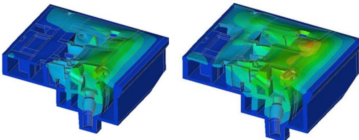
**Figure 64:** Deformation of block 1 of the plant in 2014 and 2070.
