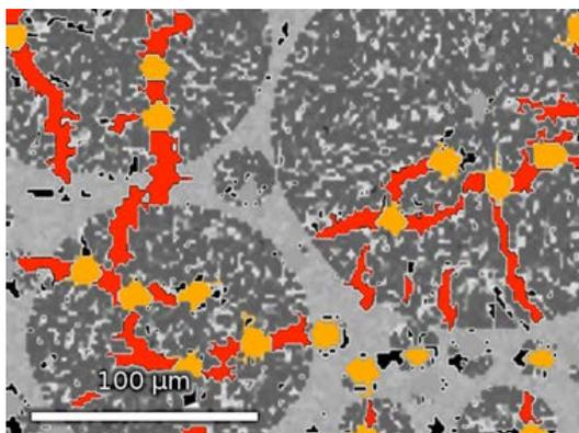
**Figure 49:** Schematic representation of the swelling process in concrete (Prof. K. Scrivener EPFL Lausanne).
