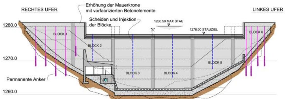
**Figure 68:** Temporary reinforcement – set-up of the vertical tension anchors.
