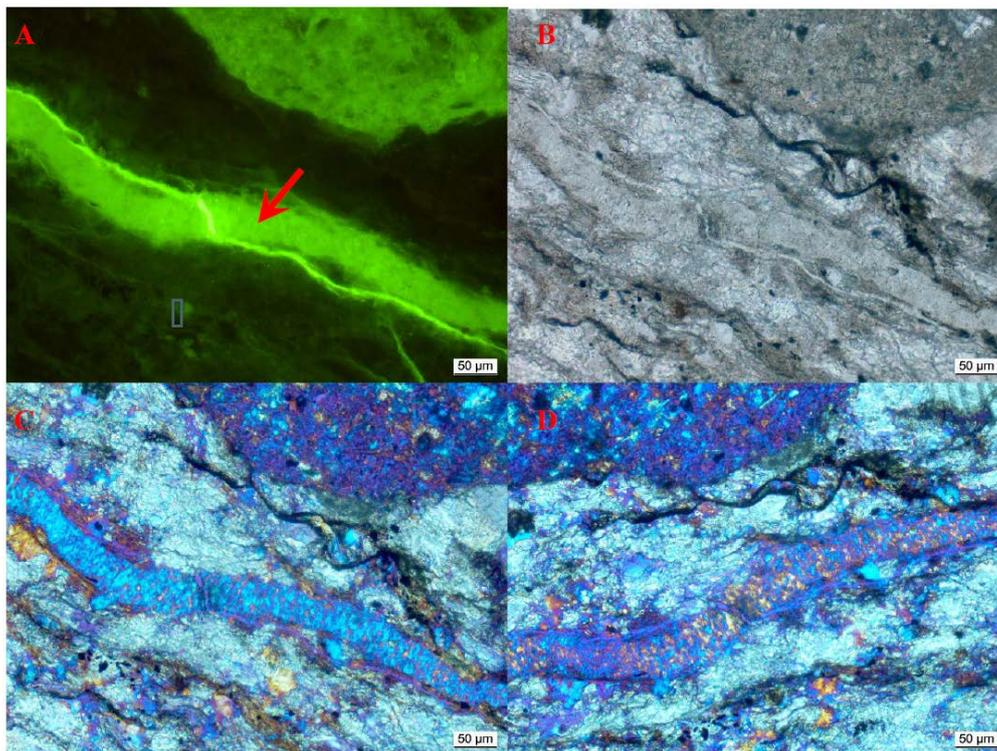
**Figure 9:** Thin section image of a crack completely filled with AAR-generated products (red arrow) in an aggregate grain under four different light conditions (A = fluorescent light, B = polarized light, C = crossed polarizing filter and plasterboard, D = same as C but rotated by 45°) [10].
