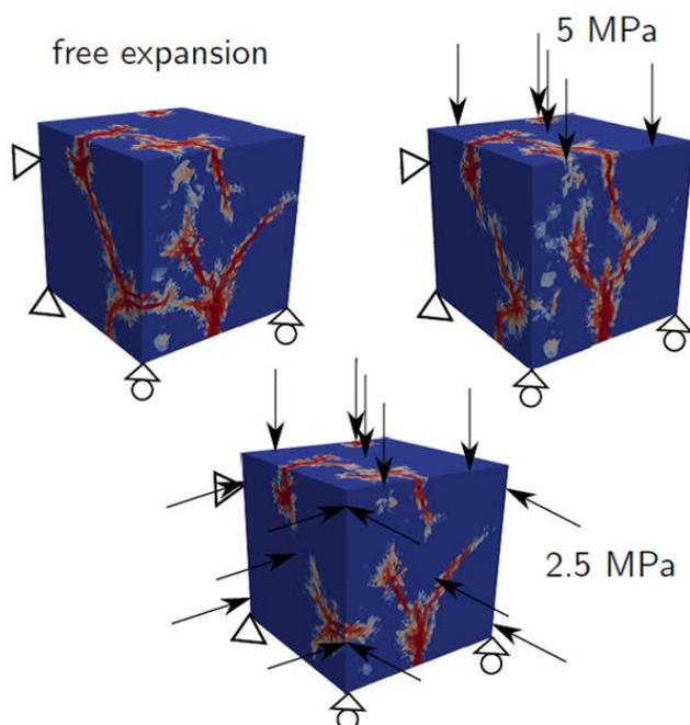
**Figure 5:** Load influence on AAR areas (red and gray) due to numerical 3d-computer simulation (top left without external load, top right with single-axis compressive load, and below with three-axis compressive load) [9].
