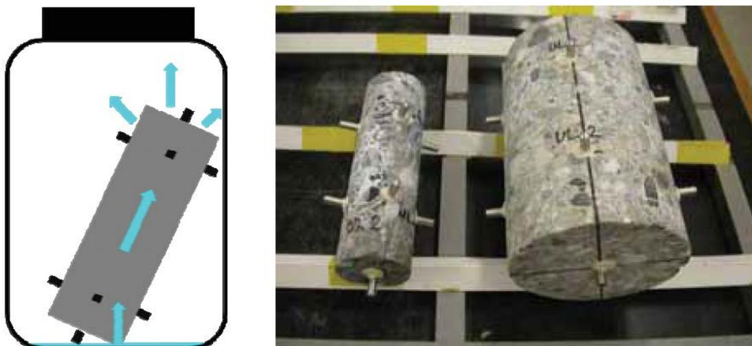
**Figure 20:** Cores for AAR residual swelling determination [5].
