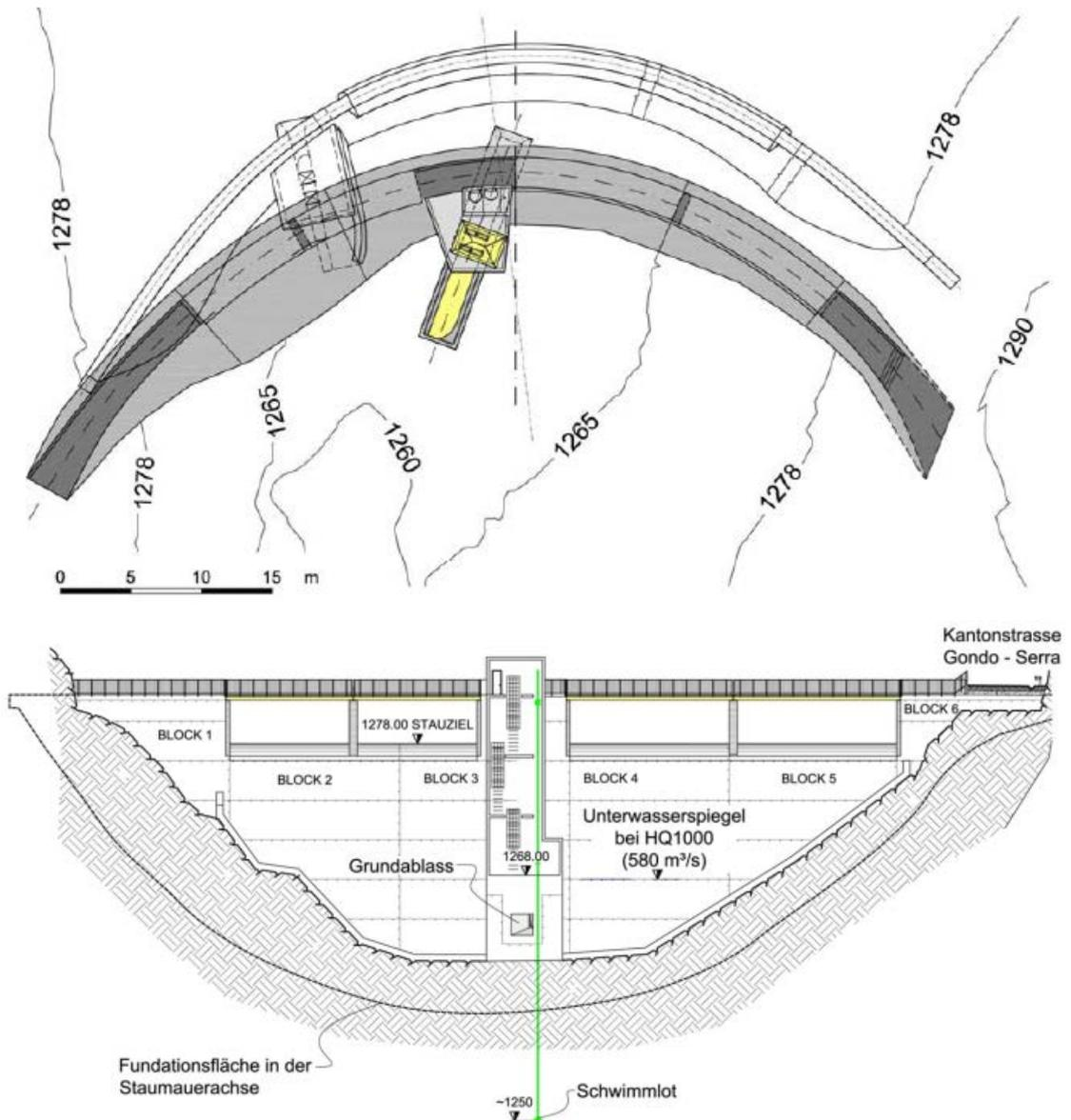
**Figure 70:** Plan view and new Sera dam raise.
