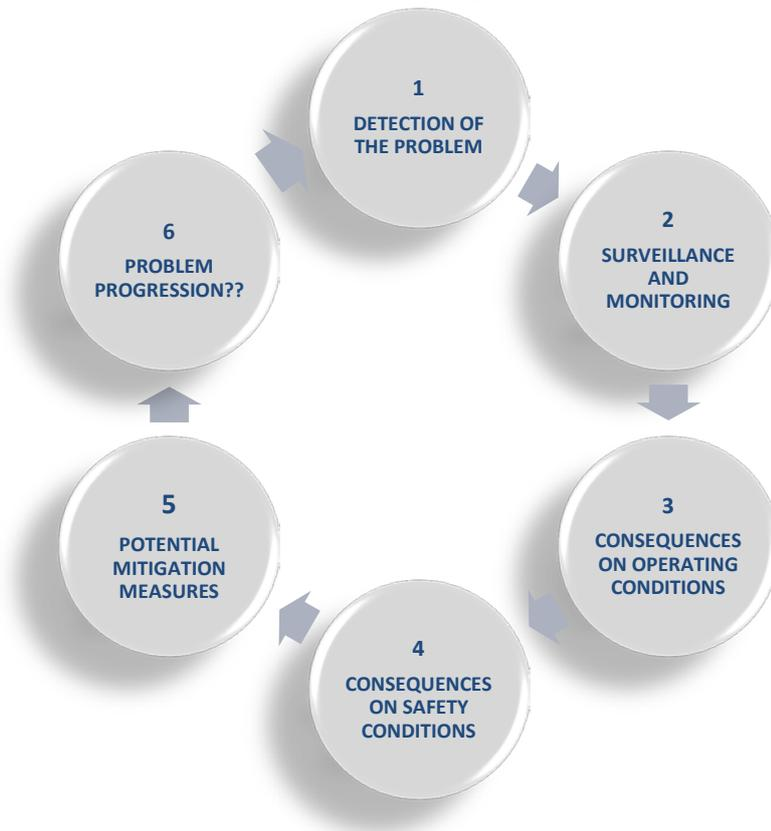
**Figure 82:** Typical monitoring cycle of a dam affected by concrete swelling.
