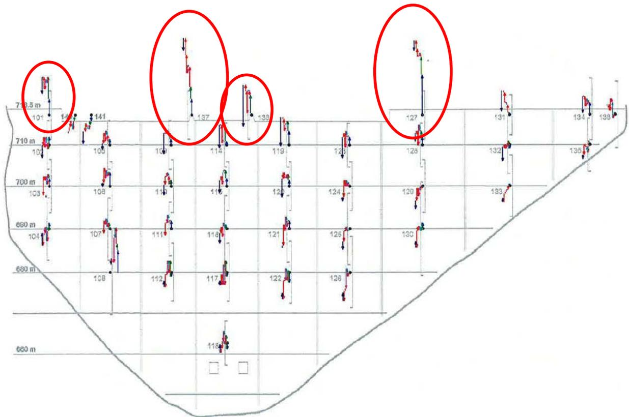
**Figure 53:** Displacements of the measurement points at the downstream face (1984–2008).
