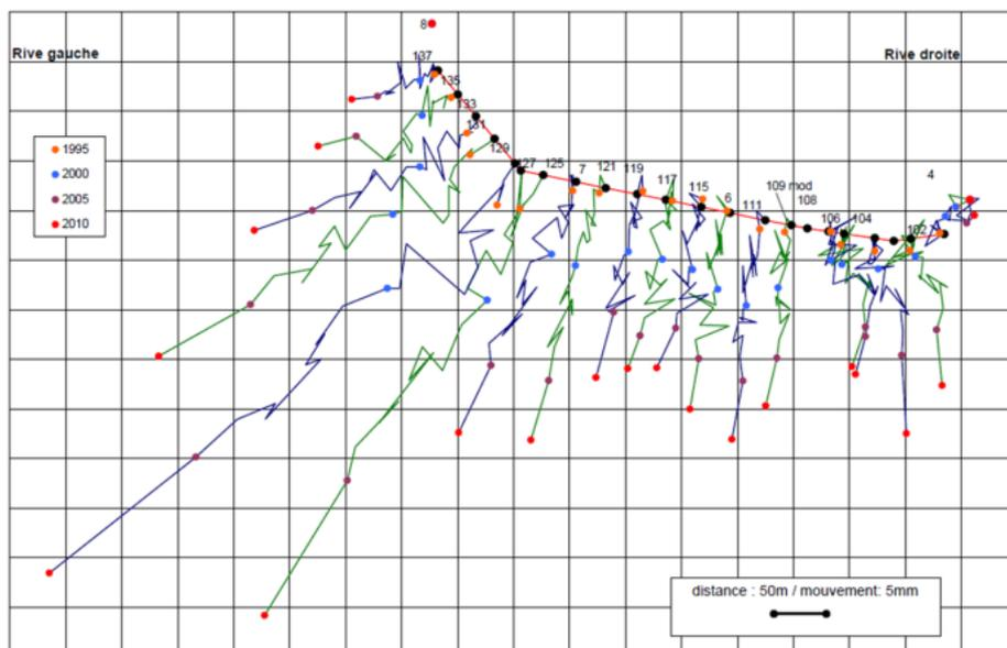
**Figure 76**: Planimetric crest displacements through geodetic measurements .
