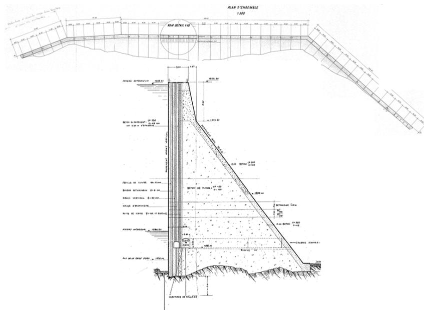
**Figure 74:** General plan view and vertical cross section of the Salanfè Dam.
