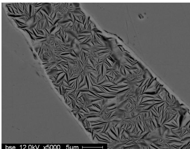
**Figure 10:** Electron micrograph (REM // SEM) image of a micro-crack filled with AAR generated products in the gneiss aggregate sample of a dam [10].
