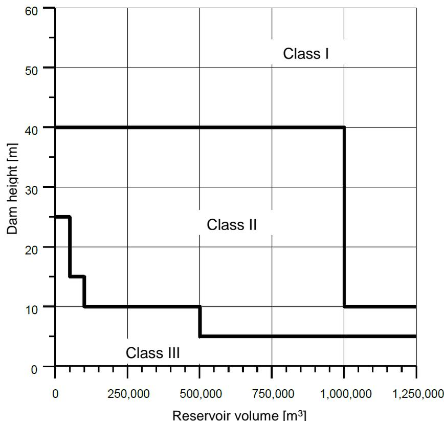
**Figure 23:** Definition of the three different dam classes.
