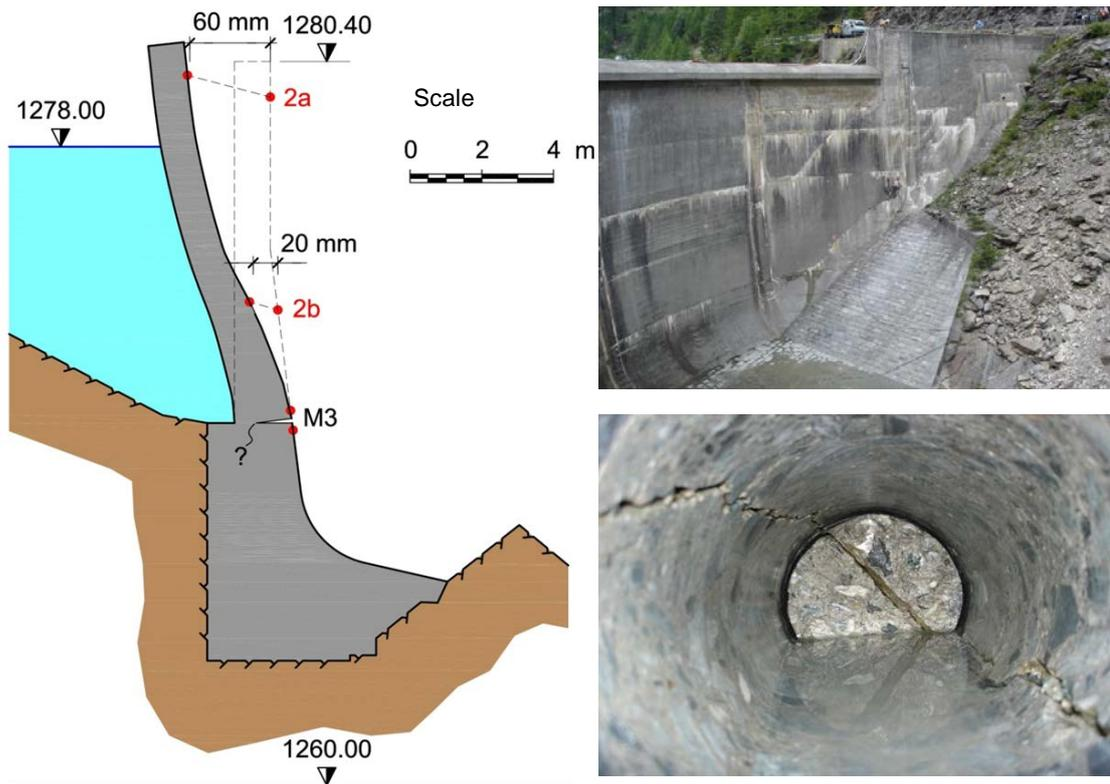
**Figure 67:** Cross section of vertical displacement towards upstream – development of cracking at the dam base.
