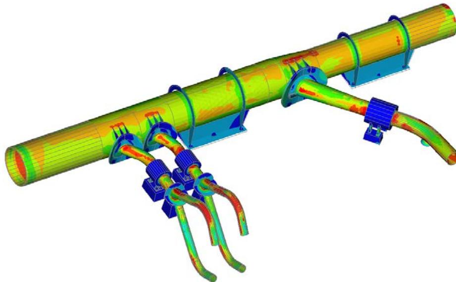
**Figure 65:** Stress state of the load distributor and the pipes of the group 1 calculated from AAR-generated deformations.
