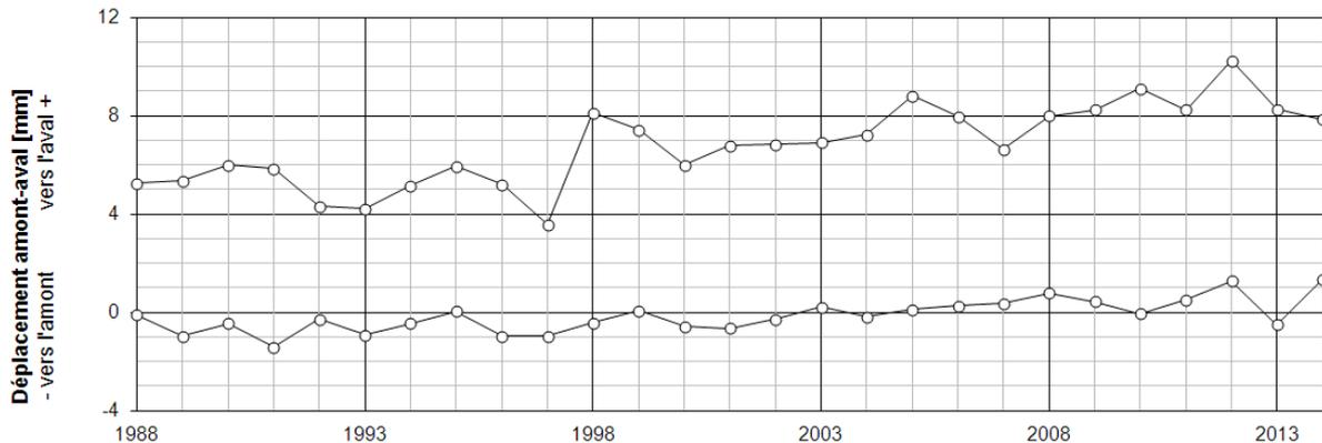
**Figure 59:** Extreme displacements (min and max) upstream-downstream of the central pendulum.
