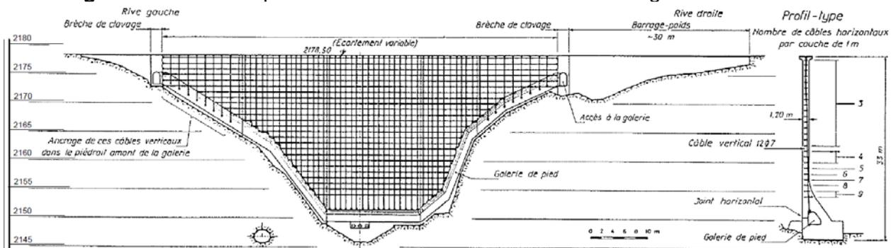
**Figure 57:** Upstream view showing the network of pre-stressed cables in the arch section.
