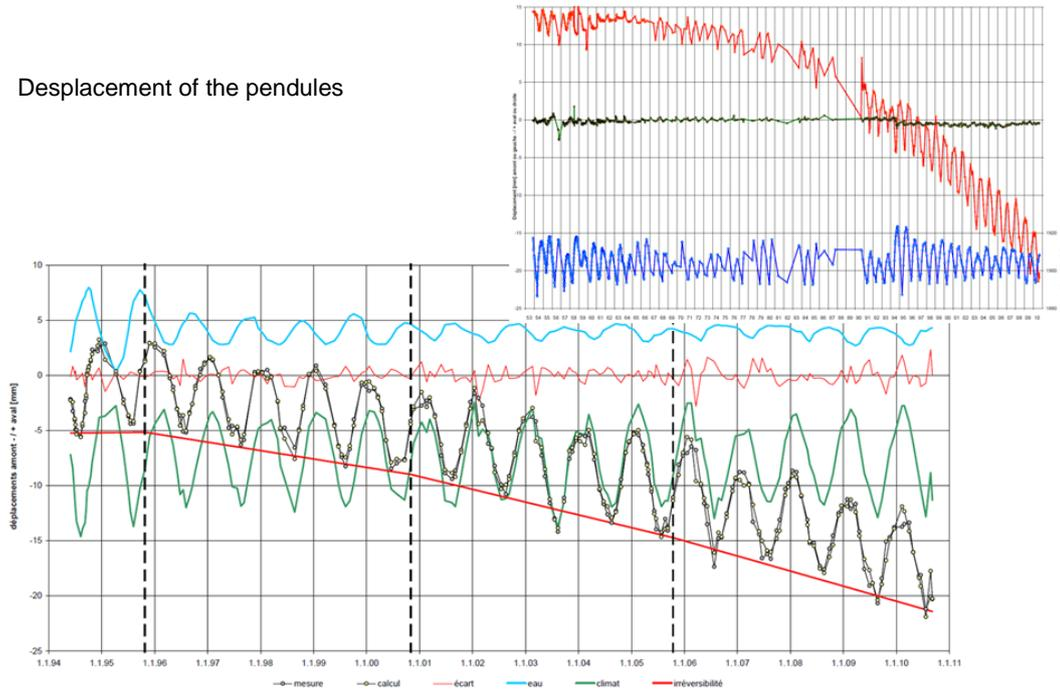
**Figure 75** : Longitudinal and transversal displacements. Statistical analysis of the pendulum behavior.
