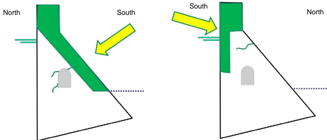
**Figure 47:** Greater swelling in sun-facing concrete areas, and places of first structural crack occurrence.
