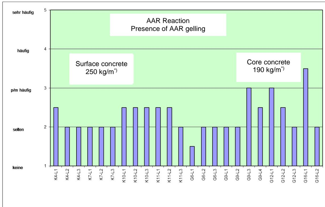
**Figure 45:** Description of the occurrence of AAR gelling for 2 cement dosages in the same dam.
