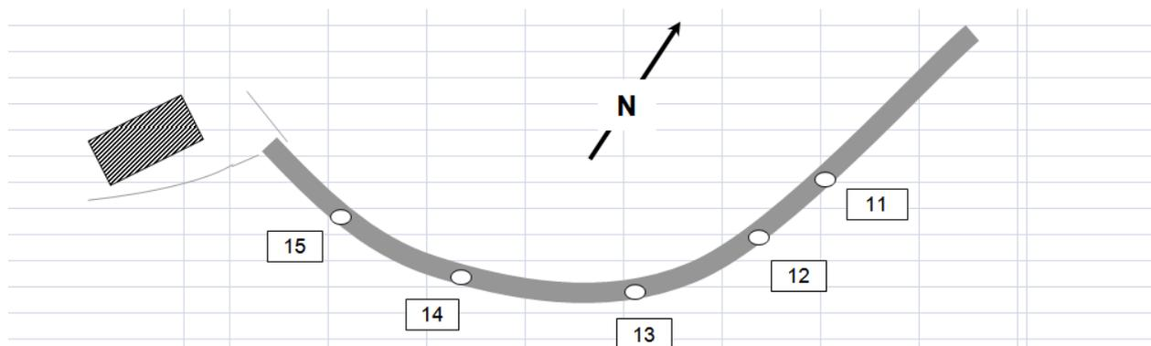
**Figure 60:** A quasi-linear evolution of displacements of various leveling points makes it possible to estimate the rate of displacement relative to the maximum height of the dam structure at  $10.3 \mu\text{m}/\text{m}/\text{year}$ .
