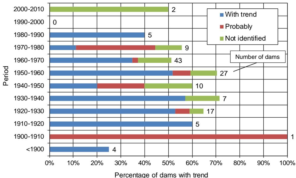
**Figure 32:** Percentage of dams affected by trends according to construction period.
