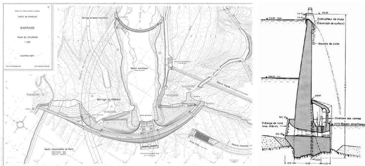
**Figure 52:** Plan view and cross section of the Châtelot Dam.
