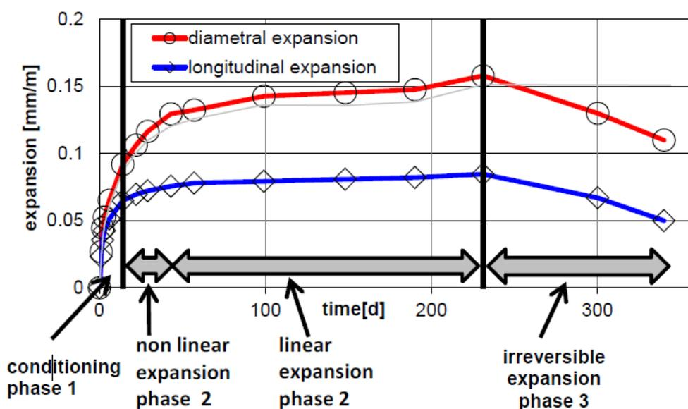
**Figure 21:** Diametral expansion (= red curve) and longitudinal expansion (= blue curve) [10].
