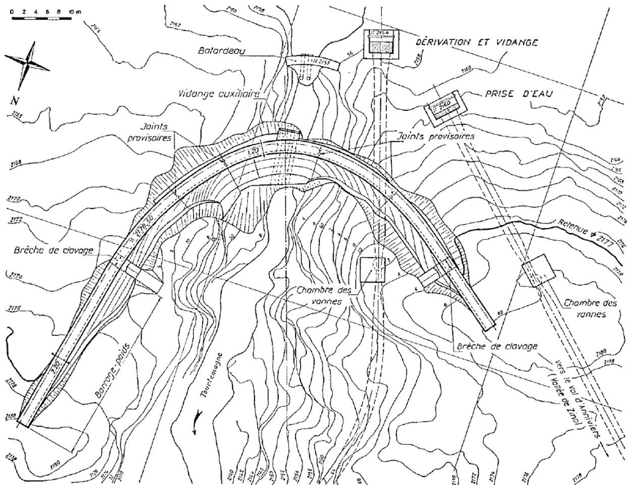
**Figure 56:** General plan view of the Tourtemagne Dam layout.
